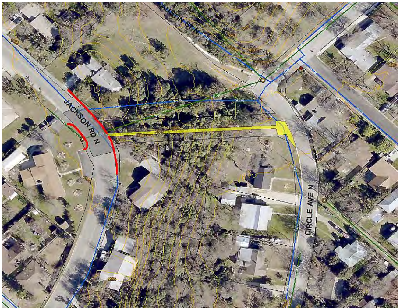
Figure 73 – Conceptual Drainage Chute at Circle Avenue
