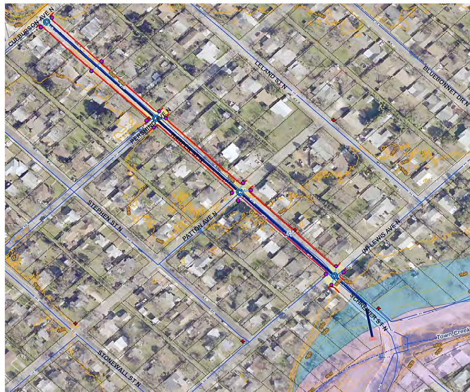
Figure 72 – Conceptual Street Drainage Improvements at Harper Street
